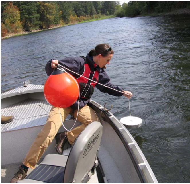
figure 2.2. Setting targets from the McKenzie Fire and Rescue jet boat on river before the flight. The targets are cement discs painted white for visibility in the image.
