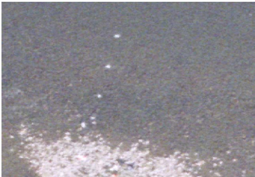
figure 2.3. True colour image at the river's edge zoomed-in 13X relative to figure 2.4 to illustrate image speckle and granularity. The white objects in the river are ground targets placed in the water at varying depths. Pixel resolution is approximately 10 cm.
