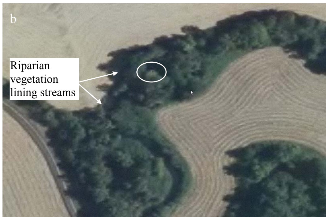
Figure 4.10. Difficulties in evaluating small dam impacts on stream morphology. In the 0.5 m resolution OIE images, riparian vegetation partially blocks views of the river even in more sparsely vegetated ecoregions like the Eastern Cascades ecoregion (a). In agricultural regions, forest stream buffers can obscure the majority of channel, as in this example from the Willamette Valley (b). Small dam locations are circled.
