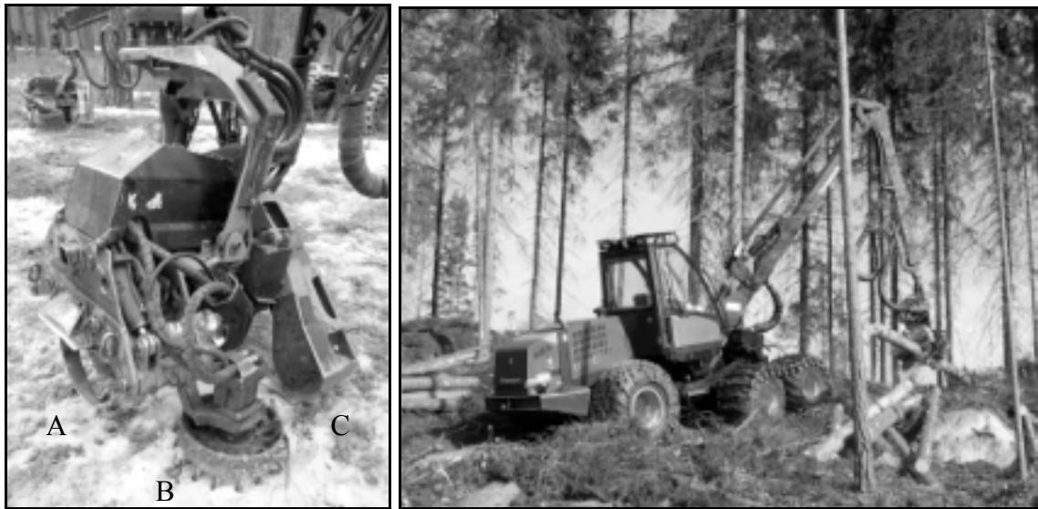
Figure 5. Harvester. (Left) cutting-head elements: (A). de-limbing knives (B). feed rollers (C). grappling arms with chainsaw. (Cutting-head is oriented horizontal to the ground here.) (Right) Harvester de-limbing logs in the field. Photo: www.wikimedia.org
