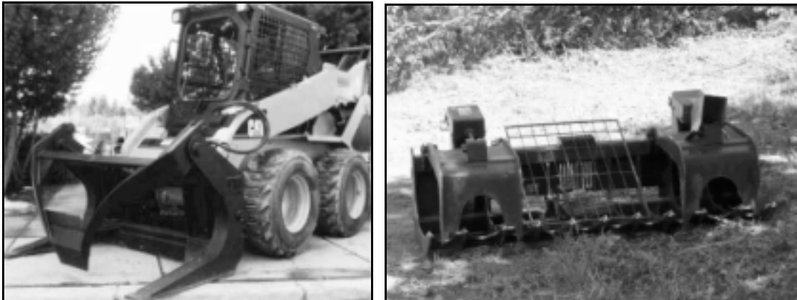
Figure 8. (Left) Skid-steer tractor with grapple fork attachment. Photo: ekf-industries.com. (Right) Grapple fork attachment for fine material.
