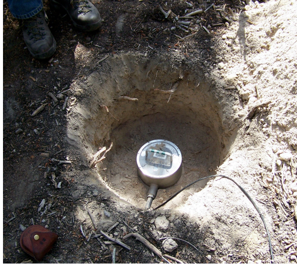
Figure 10. L-22D seismometer being oriented and buried in 18 inches of volcanic ash at station 33. The three channels were oriented vertically, north-south, and east-west.
