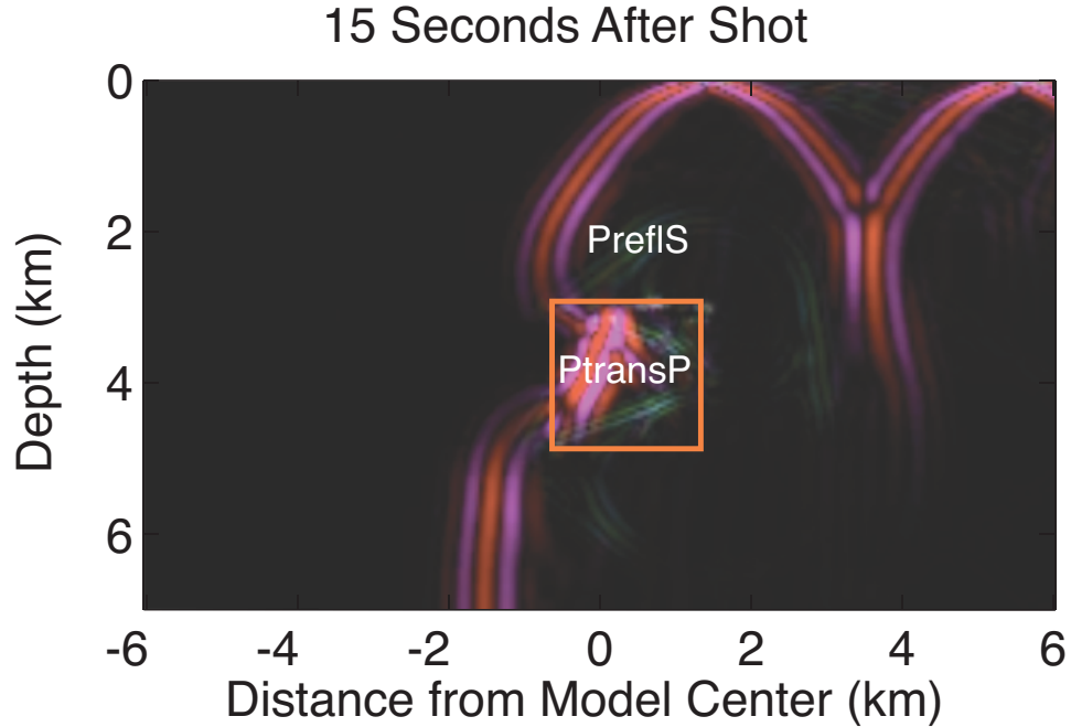
Figure 3a. Finite-difference waveforms in a velocity model with 2 by 2 km 2 low-velocity body similar to Figure 1. The P-wave in pink has been delayed and focused within the low-velocity body as a high-amplitude PtransP. A converted PreflS phase in green emerges from the top of the low-velocity body.
