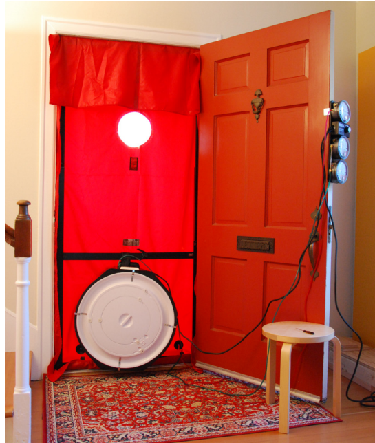
Figure 3: Blower door unit installed prior to test
