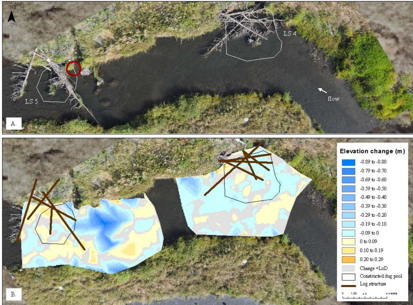
Figure 7. Log structures 4 and 5, MFJD Forrest reach a) is the log structure and rootwad orientation. Red circles indicate locations of rock spur removal and the white line delineates the original constructed dug pool. b) is 2010-2008 DEM of difference (DoD) showing elevation change (m)
