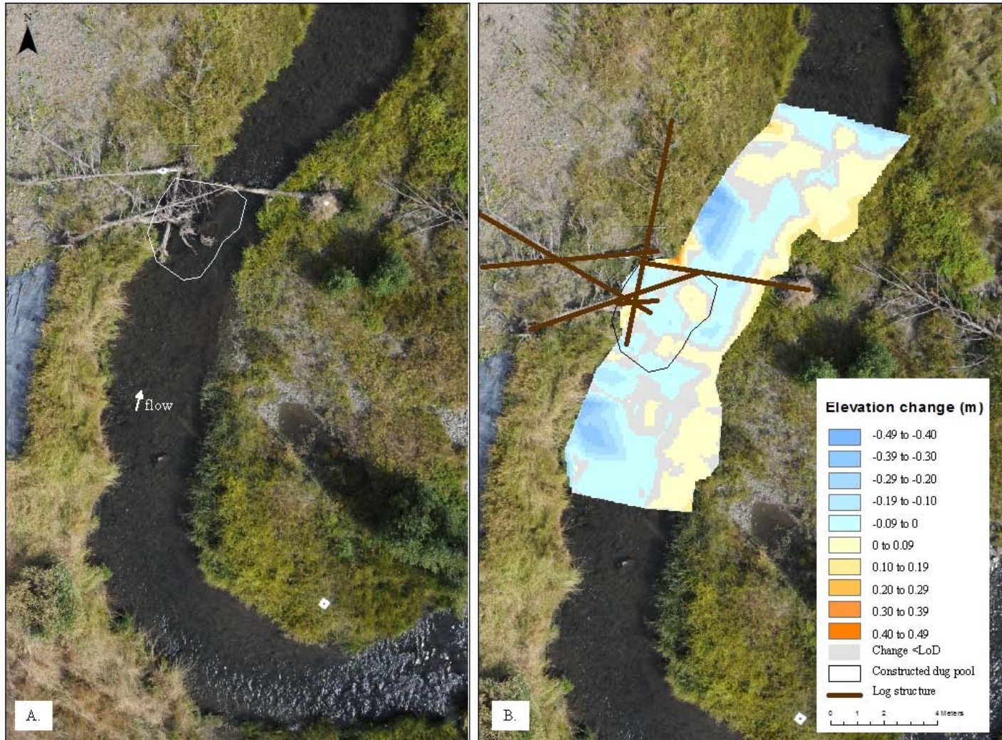
Figure 8. Log structure 8, MFJD Forrest reach a) is the log structure and rootwad orientation. The white line delineates the original constructed dug pool. b) is 2010-2008 DEM of difference (DoD) showing elevation change (m)
