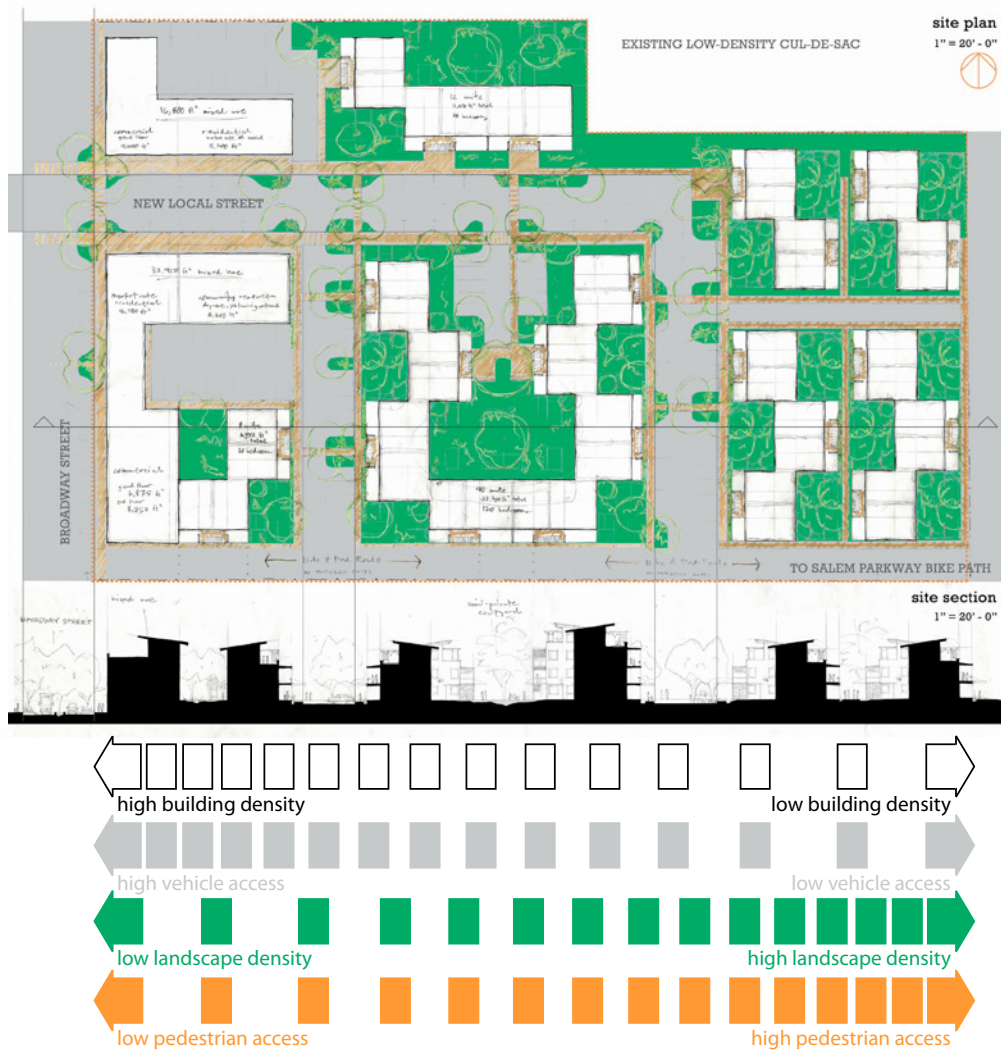
Figure 62: Orchard Village site plan and cross-section with accompanying site gradient diagram showing east-west distribution of building density, landscape density, vehicle access, and pedestrian access (Shane O’Neil).
