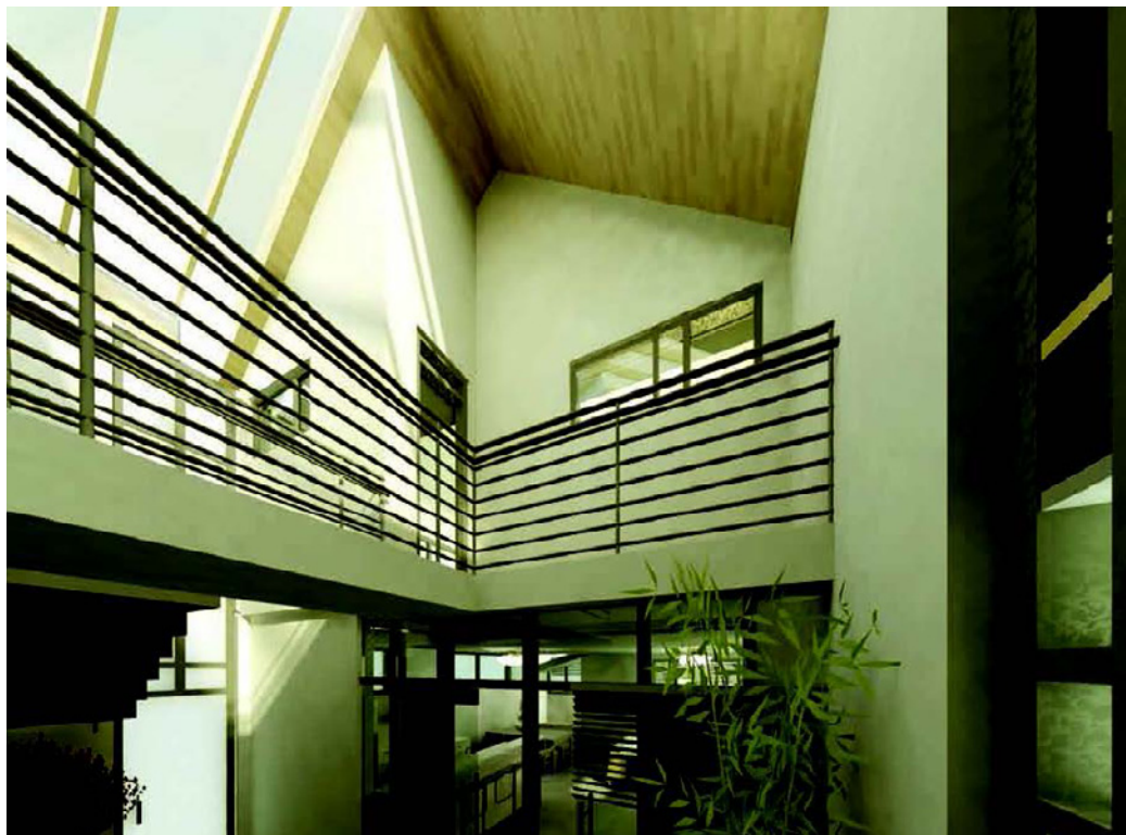
Figure 22: View of unconditioned interior courtyard with polycarbonate roof to diffuse daylight, minimize glare, and reduce heat loss in conditioned spaces (Caitlin Gilman).
