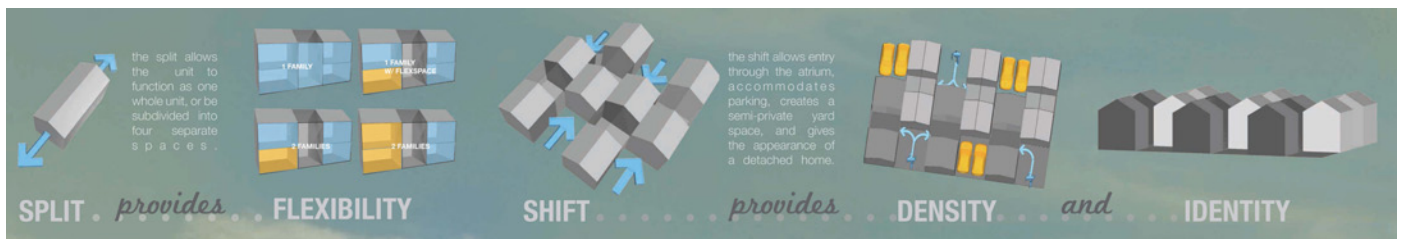
Figure 39: Diagram of how the form of the Split-Shift housing type responds to the need to design resilient housing (Caitlin Gilman).
