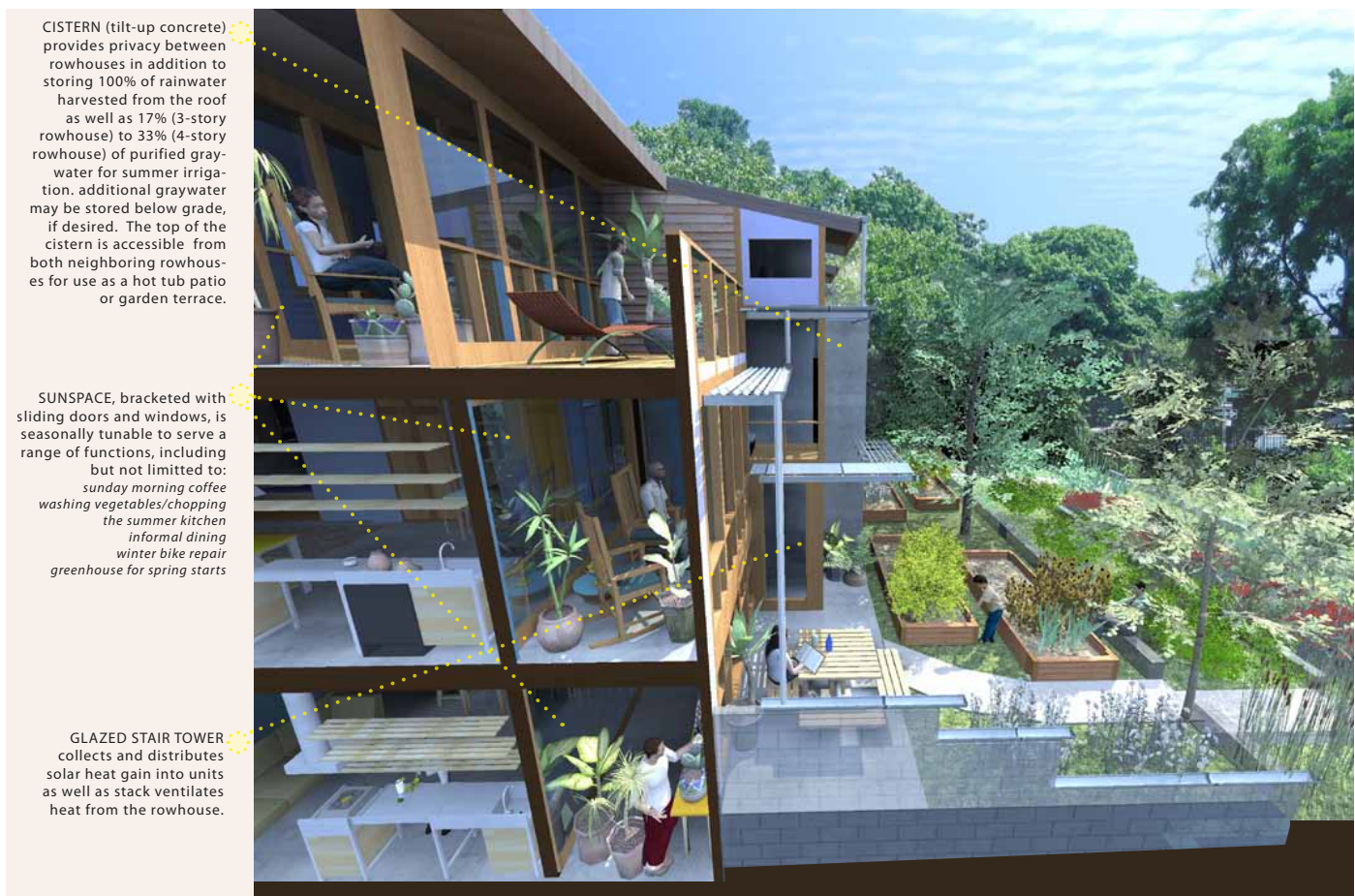
Figure 36: Cross-section view through south façade of row house, showing layers of sunspaces, shading strategies, and garden spaces (Erin Upham).
