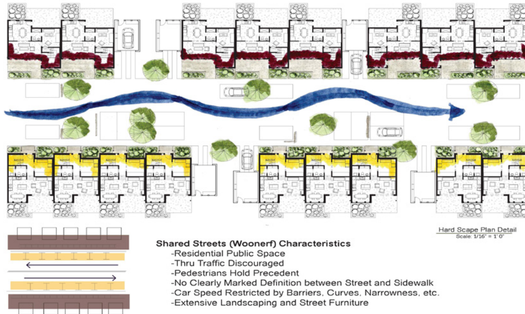
Figure 65: Diagram of residential woonerf showing traffic lane, parking spaces, and landscape elements connecting the front of the units (Ali Clark).
