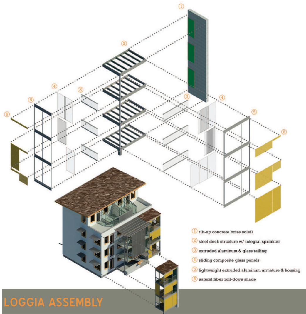
Figure 30: Diagram showing loggia assembly and layers of thermal and environmental control using occupant-controlled roll-down shades, and sliding composite glass panels (Shane O'Neil).
