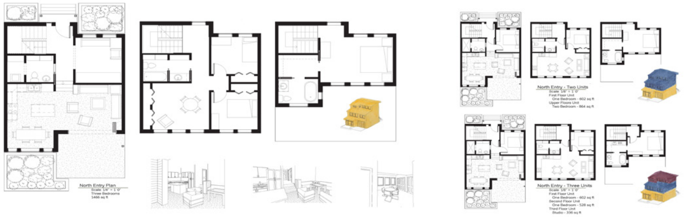
Figure 43: Plans and diagrams showing how typical two- and three-story unit can be subdivided into multiple different units as occupant needs or demographics change (Ali Clark).
