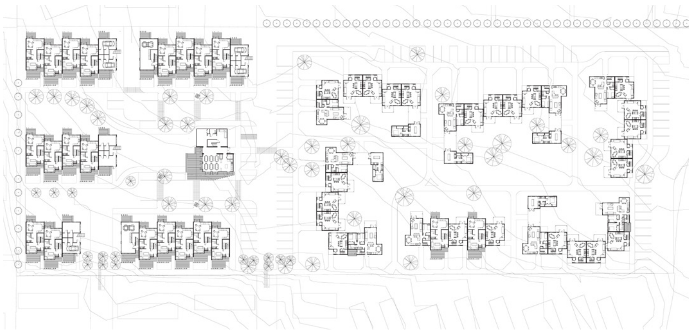
Figure 74: Proposed site layout for Meadowlark Village, including new housing and community building on the infill site and renovated existing housing with new community-use buildings (Kody Nathe).
