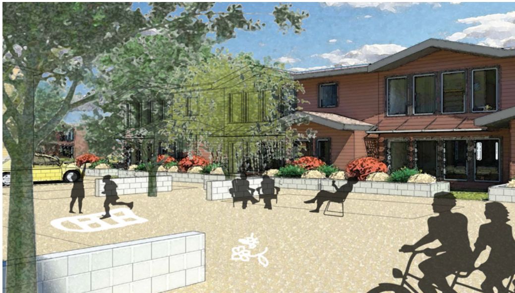
Figure 64: Exterior view showing the front entry of the units and woonerf, or “living street,” where parking, hardscaped play areas, and landscape elements slow down traffic and create an outdoor room (Ali Clark).
