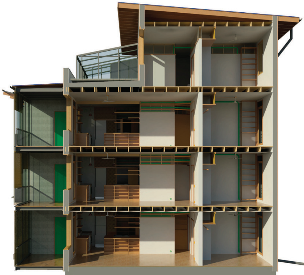
Figure 29: Cross-section perspective through unconditioned entry loggia, living spaces, and sleeping spaces (Shane O’Neil).
