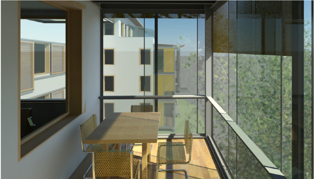
Figure 21: View from entry loggia showing layers of thermal, acoustic, and privacy controls (Shane O'Neil).
