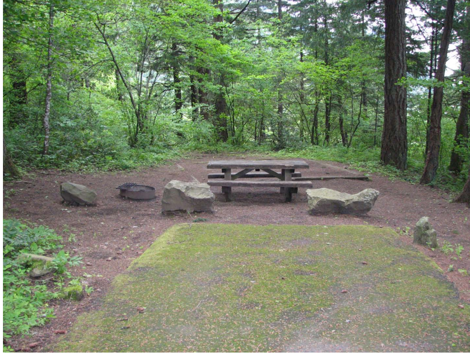
Figure 30. Example of boulders at end of garage spur. Recommend placing the boulder to the far closer to the left edge of the parking spur, to eliminate vegetation from being trampled further.
