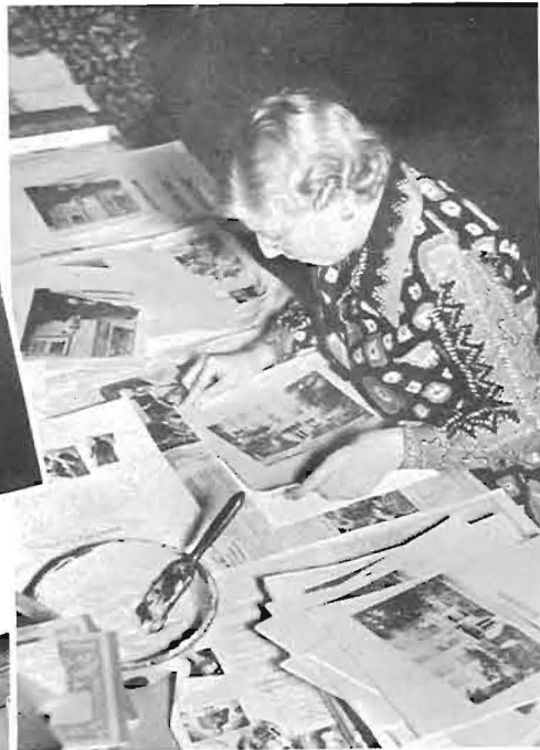
Special one and two-page color inserts must be "tipped" or glued into their respective places within the sections. This step is of necessity hand labor requiring skill and practice.
