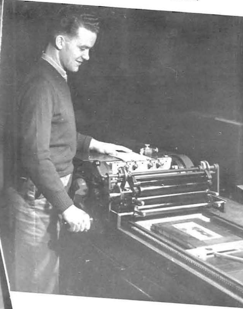
Finished "cut" is printed once in proof-press for check-up before being mounted on type-high block and sent to the big press.
