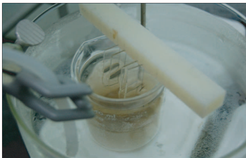
Figure 3.1. Photograph of Tollen's film fabrication setup with samples suspended in the Tollen's reaction solution. The photograph was taken within 1 minute after the start of deposition as indicated by the yellowing of the solution.
