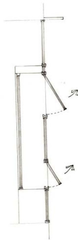
Figure A.2. Section drawing of the outside window operability.
