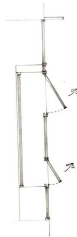
Figure 6.29. Exterior hopper windows serve as ventilation
