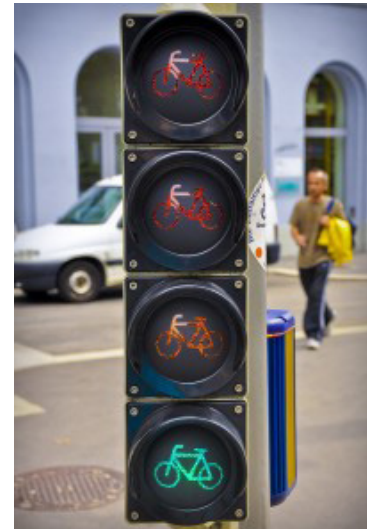
Figure 4: Bicycle traffic lights can help further separate cyclists from auto drivers by creating different times of intersection crossing.
