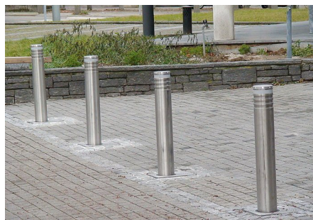
Figure 18: Remotely Retractable Bollards.
