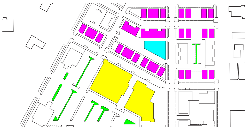
Figure 67: A diagram of sustainable strategies utilized by Approach 4; pink highlights passive solar orientation, blue highlights the community garden, yellow highlights building reuse, and green highlights bioswale placement on site.
