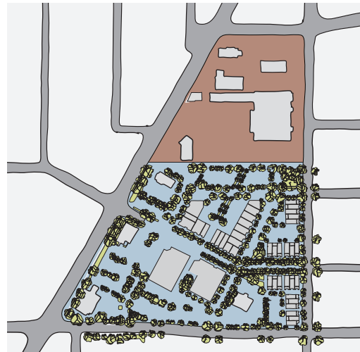
Figures 24 and 25: Impervious surfaces (brown) converted to pervious asphalt (blue) and vegetation.
