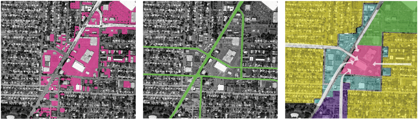
Figures 68-70: Diagrams used by Approach 5 to explore the opportunities like the continuation of green streets (shown in green in Figure 69) and constraints like the sea of parking on and around the site (shown in pink in Figure 68), as well as how the surrounding uses can influence the site and make it a central node of the neighborhood (in Figure 70, The Mohawk site is shown in pink, medical use in purple, local commercial in blue, chain retail in green, and residential in yellow).
