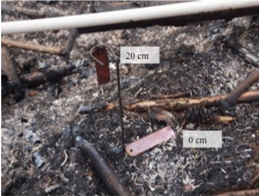
Figure 2. Temperature Sensitive Paints Set Up – Replicated twice in each plot for a total of 4 tags per plot (two at 20 cm, two at 0 cm).
