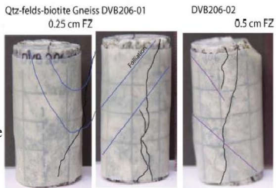
Figure 52: Tensile strength tests (above) and uniaxial compression tests were conducted. The results (graph) reveal the pegmatite has the highest rock strength and the widest fracture zone (FZ). This strengthens the field hypothesis that gouge thickness is a function the physical grain size reduction rate. The hypothesis is not robust and needs more testing.
