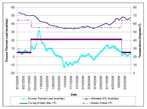
Figure 9-23: Excess Thermal Load Discharge to Silver Creek
