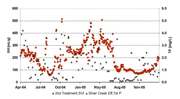
Figure 7-5: Silverton WWTP Relationship of SVI and Effluent Total Phosphorus
