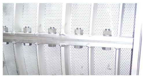
Figure 9-18: Typical Screw Press Screen
