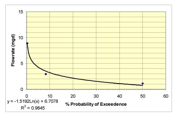
Figure 4-4: Plot of Average Annual flow, MMWWF (Method 2) and PDAF (Method 2) vs. % Probability of Exceedence per DEQ Methodology for Determining PIF.
