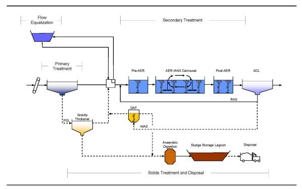
Figure 7-2: Unit Process Flow Schematic
