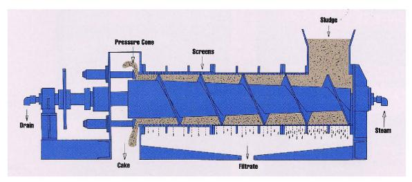
Figure 9-17: Cross-Section Schematic of Screw Press
