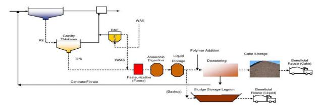
Figure 9-19: Process Schematic, Solids Processing – Alternative 1
