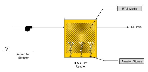
Figure 9-2: Schematic of IFAS media pilot test
