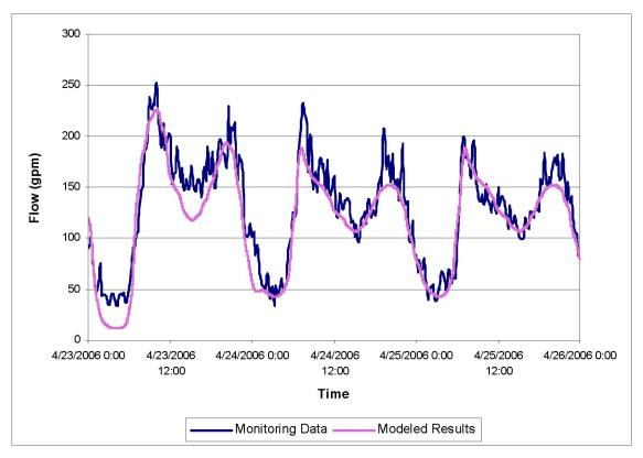
Figure 8-4: Dry Weather Flow Model Calibration
