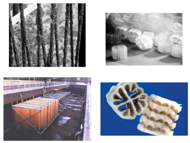
Figure 9-1: Examples of IFAS Hybrid media system
