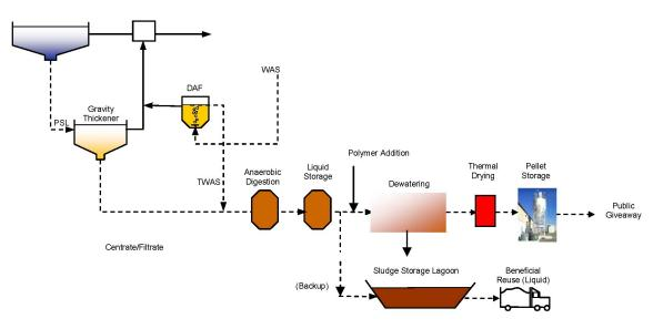
Figure 9-22: Schematic of Solids Processing Alternative 3
