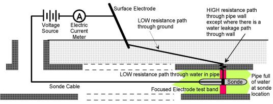
Figure 6-2: Electro-Scan Electrical Schematic
