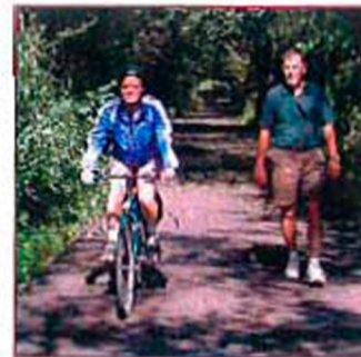
Figure 40. Trail width should accommodate concurrent, shared uses
