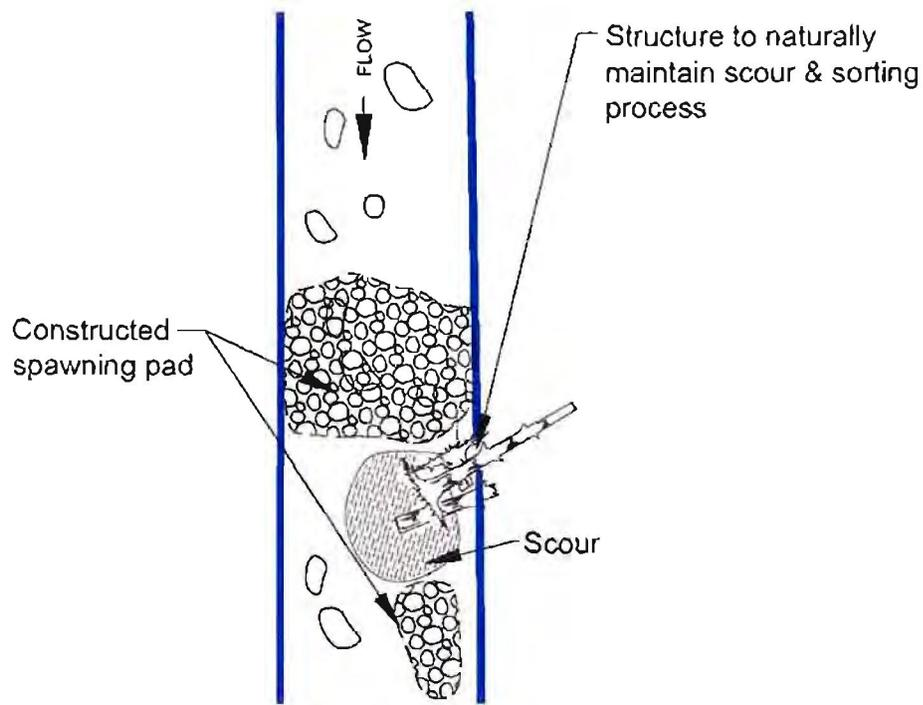
Figure 23. Conceptual drawing of gravel placement (WDFW, 2004).
