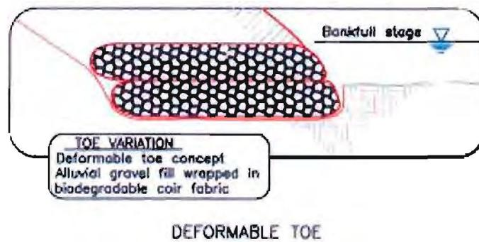
Figure 14. Conceptual drawing of roughened rock toe treatments (WDFW 2003).
