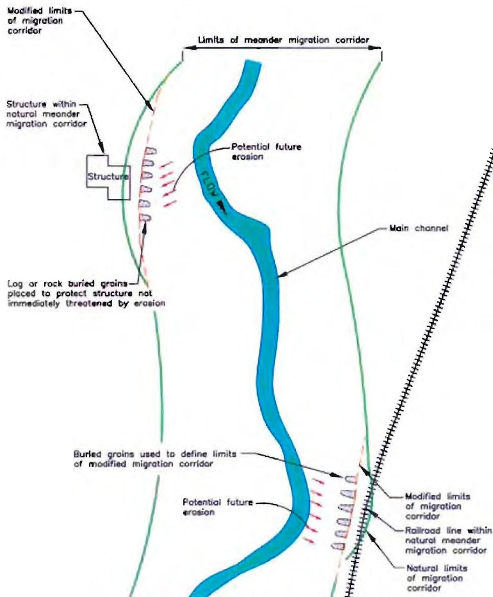
Figure 10. Conceptual drawing of setback berms used to increase the width of the stream corridor and floodplain (WDFW, 2003).
