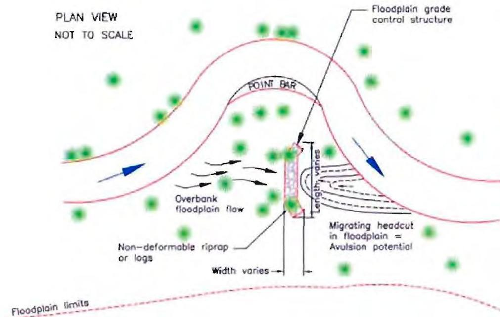
Figure 19. Conceptual drawing of floodplain grade control.
