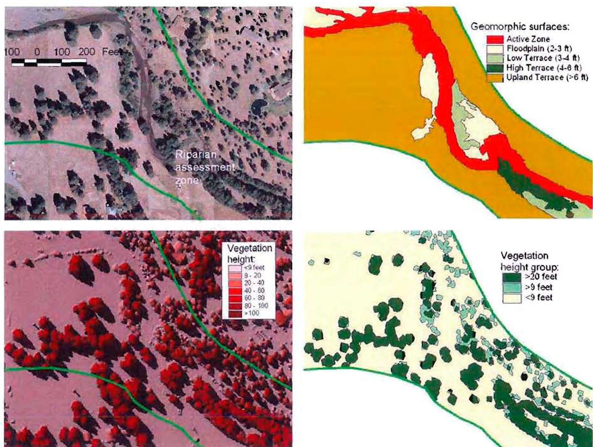
Figure 21. Example of geomorphic surfaces and vegetation heights derived from LiDAR data. This segment (Segment 3A) represents the closest example of a reference reach for the riparian condition and geomorphic surface interaction.
