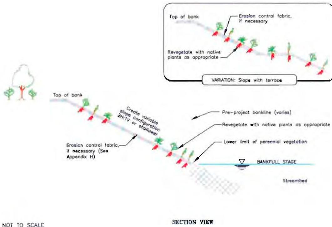
Figure 13. Conceptual drawing of bank reshaping and revegetation (WDFW 2003).
