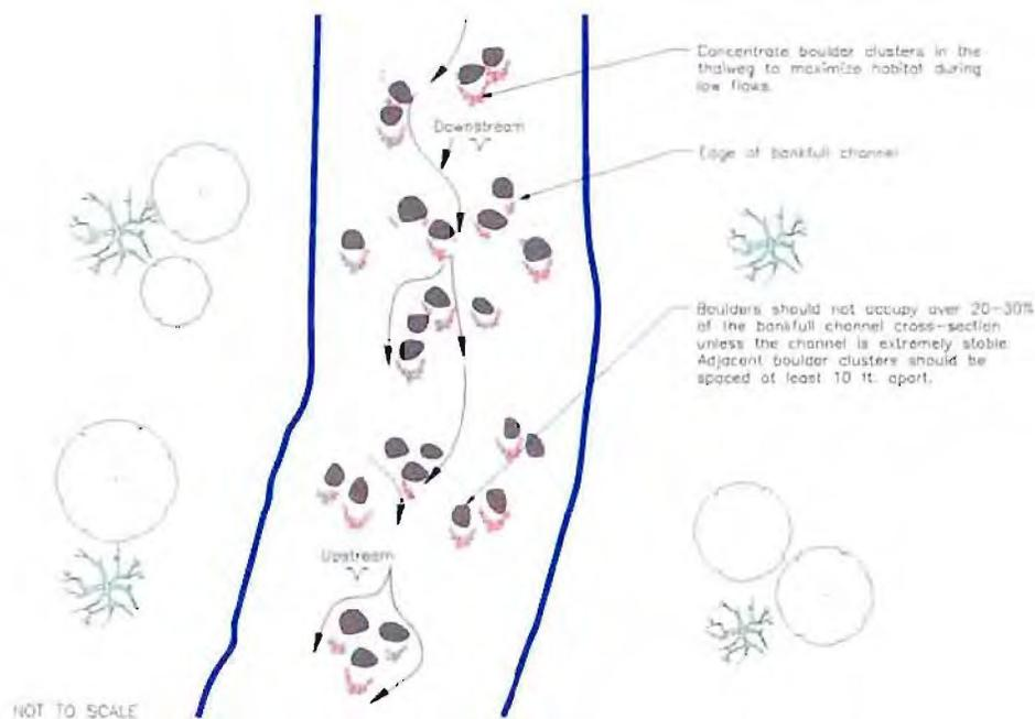
Figure 8. Conceptual drawing of boulder placement (WDFW, 2004).
