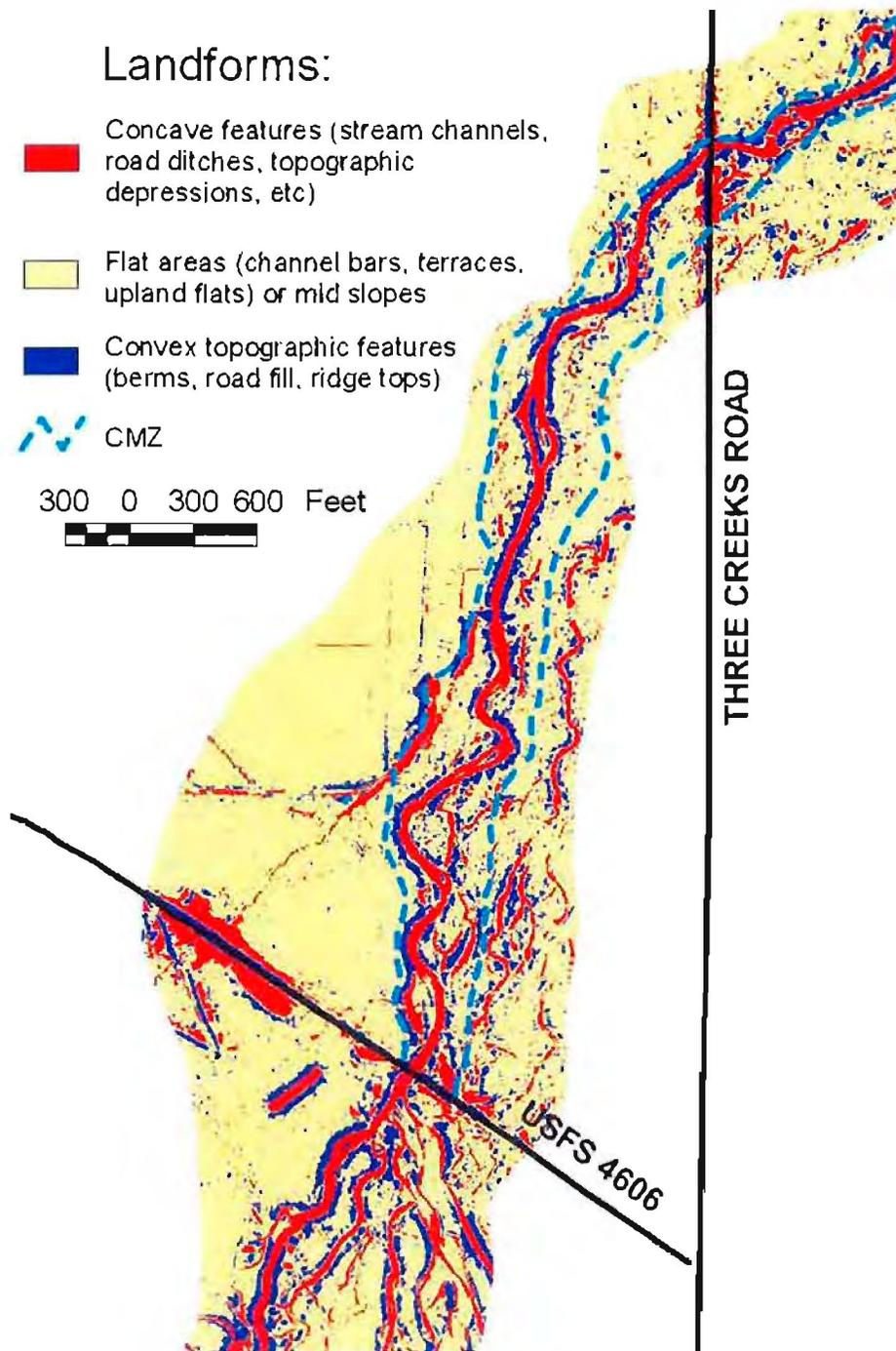
Figure 3. Example of landforms and channel migration zone delineation at upstream end of project area.
