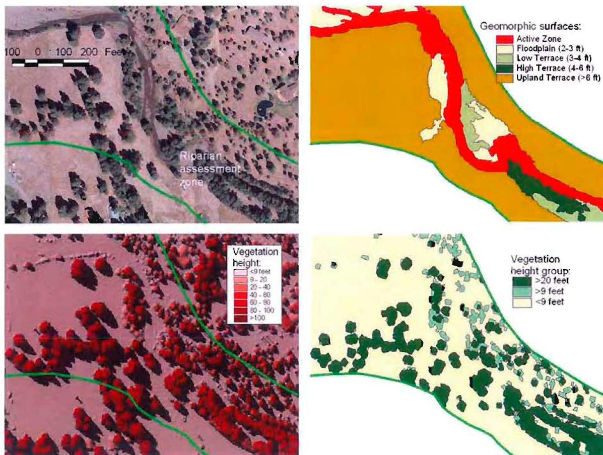
Figure 5. Example of geomorphic surfaces and vegetation heights derived from LiDAR data. This segment (Segment 3A) represents the closest example of a reference reach for the riparian condition and geomorphic surface interaction.
