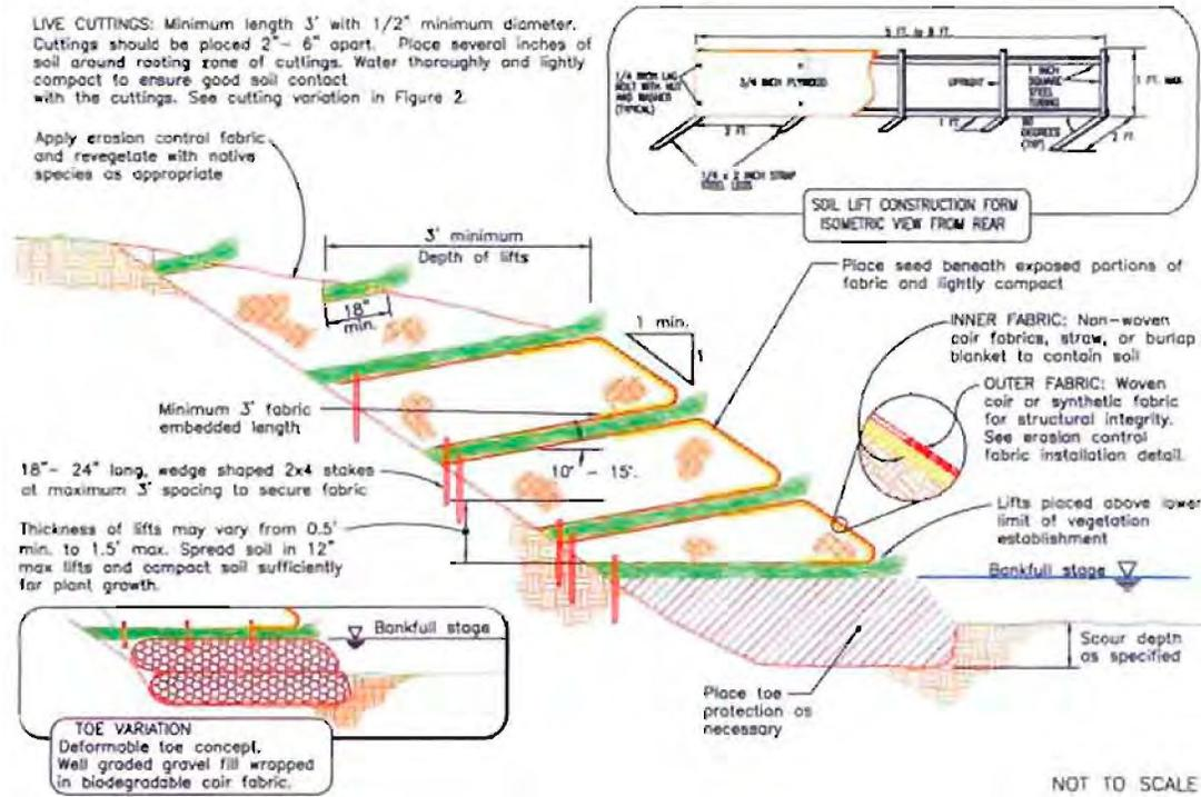
Figure 12. Soil reinforcement through the use of live cuttings (WDFW, 2003).
