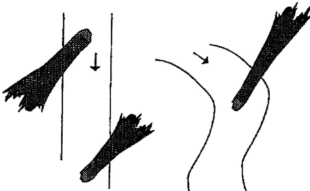
Figure 7. Conceptual drawing of large woody material placement (ODF, 1995). Pieces placed diagonal to flow can direct flow away (left) or towards (middle) bank. Pieces placed on meander bends (right) can enhance scour.
