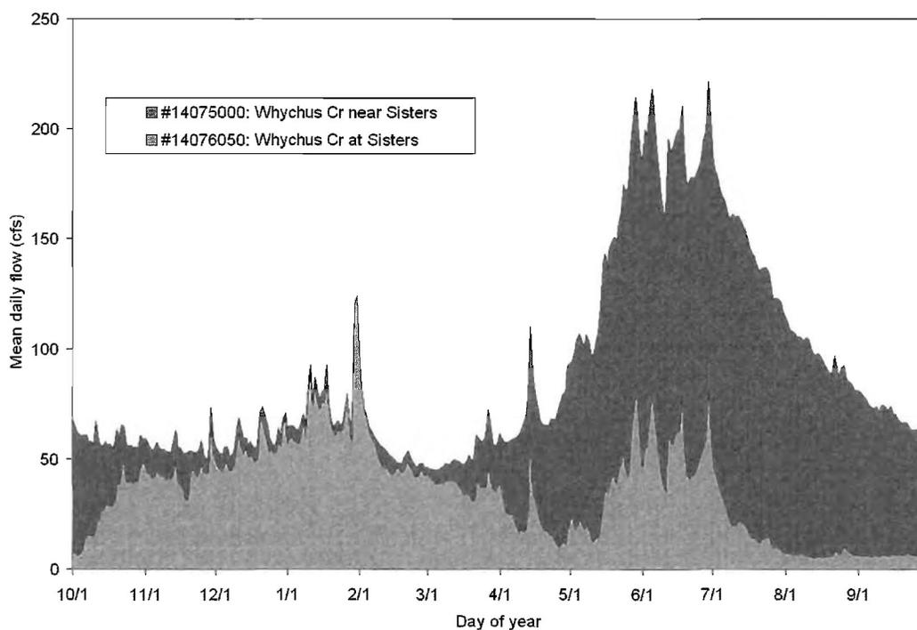
**Figure 4. Mean daily flow comparison for the period 5/2000 - 9/2006 upstream of the TSID diversion (gage #14075000) and within the project reach (gage #14076050).**
