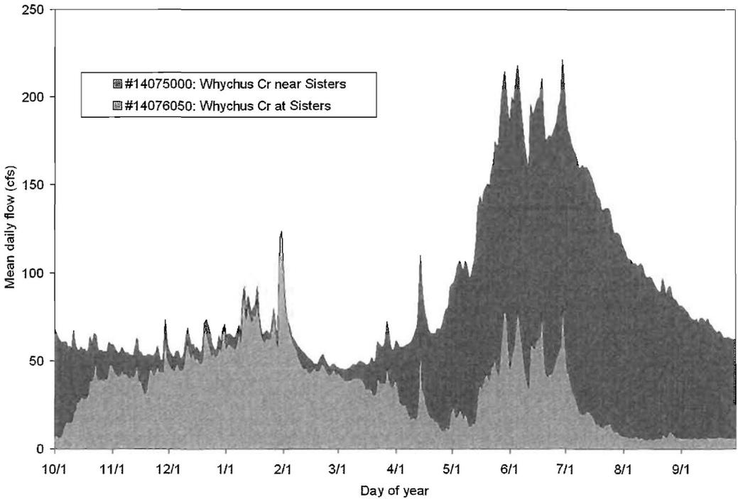
**Figure 8. Mean daily flow comparison for the period 5/2000 - 9/2006 upstream of the TSID diversion (gage #14075000) and within the project reach (gage #14076050).**
