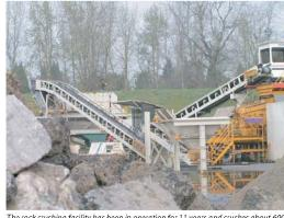
The rock crushing facility has been in operation for 11 years and crushes about 600 tons of concrete and asphalt a month.
