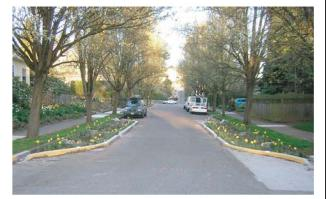
AFTER: Landscaped stormwater curb extensions reduce the amount of stormwater that flows off Siskiyou Street into the combined sewer system. Stormwater flows into the landscaped areas through breaks in the curb and soaks into the ground. The curb extensions are landscaped with plants that help filter pollutants.
