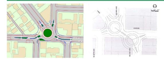
Three options were forwarded to the April 2 Open House – Alternative A: Minor signal changes and pedestrian improvements; Alternative B: Remove 21st from the signalized intersection to create a new pedestrian crossing; and Alternative C: Roundabout (single or double).
