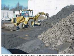
Broken concrete and aphalt are brought to the Maintenance Bureau's recycling facility, where it broken down into smaller pieces before being taken to the impact
