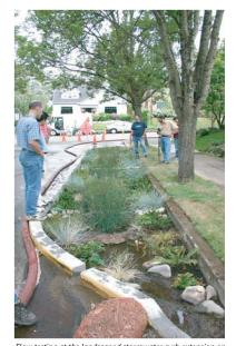
Flow testing at the landscaped stormwater curb extension on NE Siskiyou Street measures the amount of infiltration and
