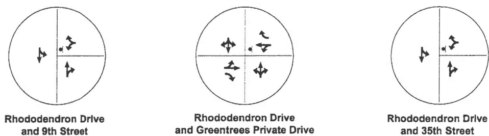
Figure1. Existing Intersection Geometry
