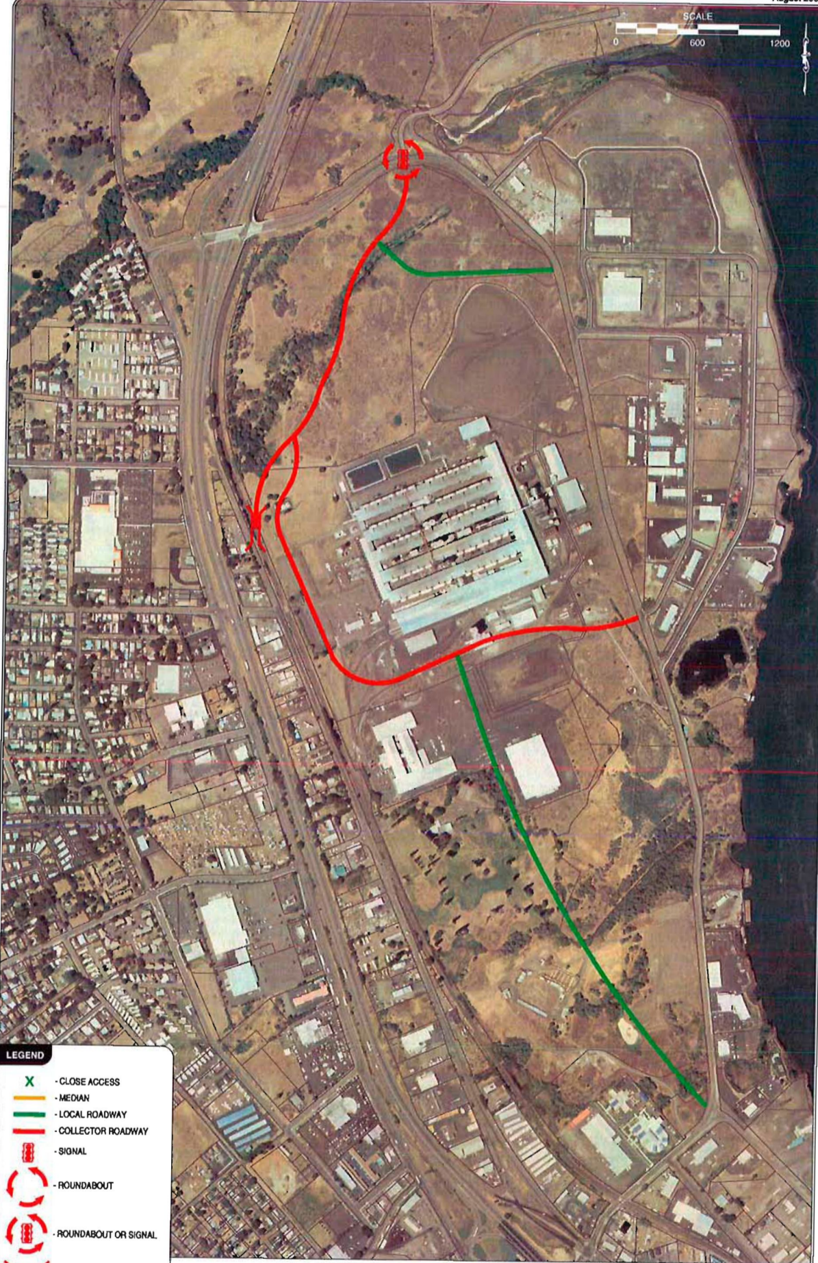
LOCAL CIRCULATION AND ACCESS DESIGN CONCEPTS CONCEPT E-3A: ONE NORTHERN GRADE-SEPERATED CROSSING OF THE UP THE DALLES, OREGON FIGURE 6-11
