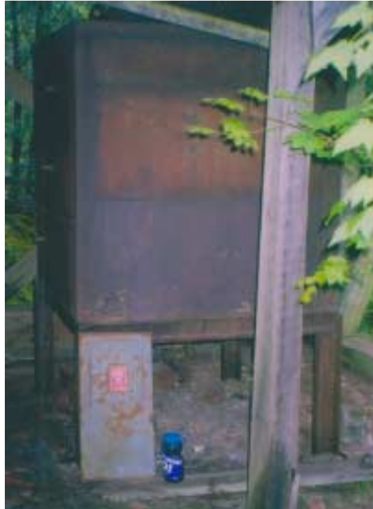
Fig. 16. Retort for roasting ore at the Kiggins Mine. Note: The photo was taken with a water bottle 8" in height included for scale. Photo by the author.
