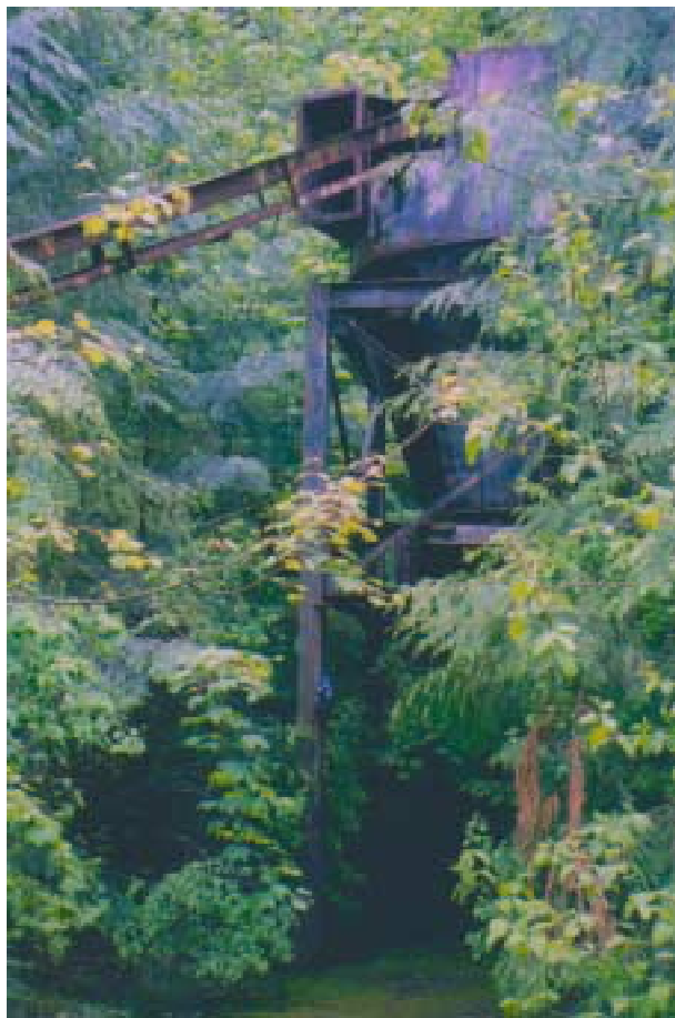
Fig. 18. Conveyor apparatus and ore hopper at the Kiggins mine. Note: The rock crusher that used to be found beneath the ore hopper was removed from the site between 2000 and 2002. Note: The photo was taken with a water bottle 8" in height included for scale. Photo by author.
