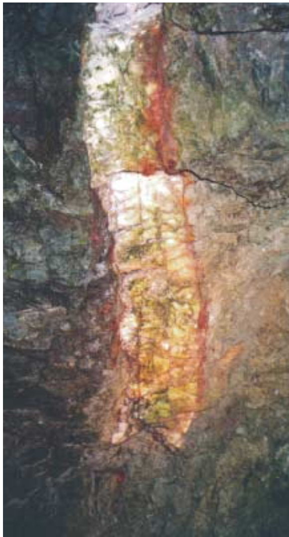
Fig. 3. Calcite vein bearing cinnabar at the Nisbet mine. Note: The white calcite vein is approx. 4" in width, and is generally encased by narrow red veinlets of cinnabar. Photo by author.
