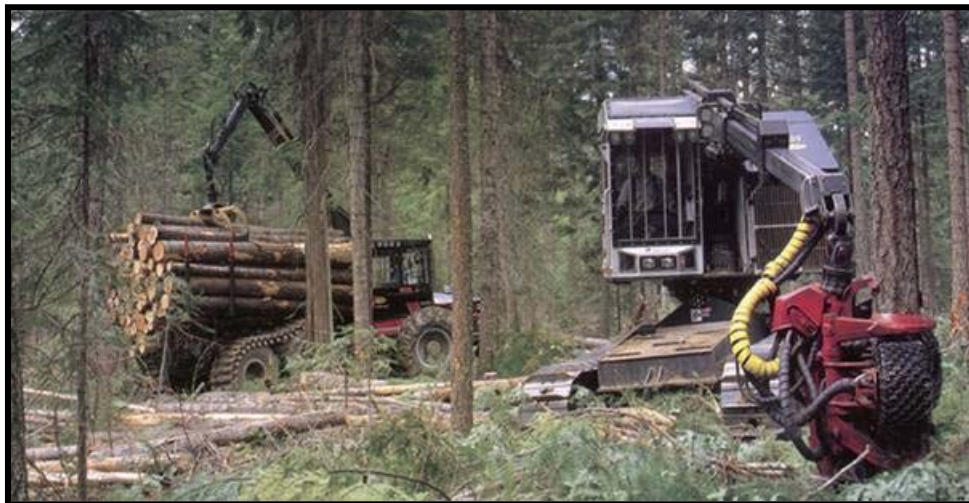
Mechanical Thinning using a cut-to-length harvesting system.
