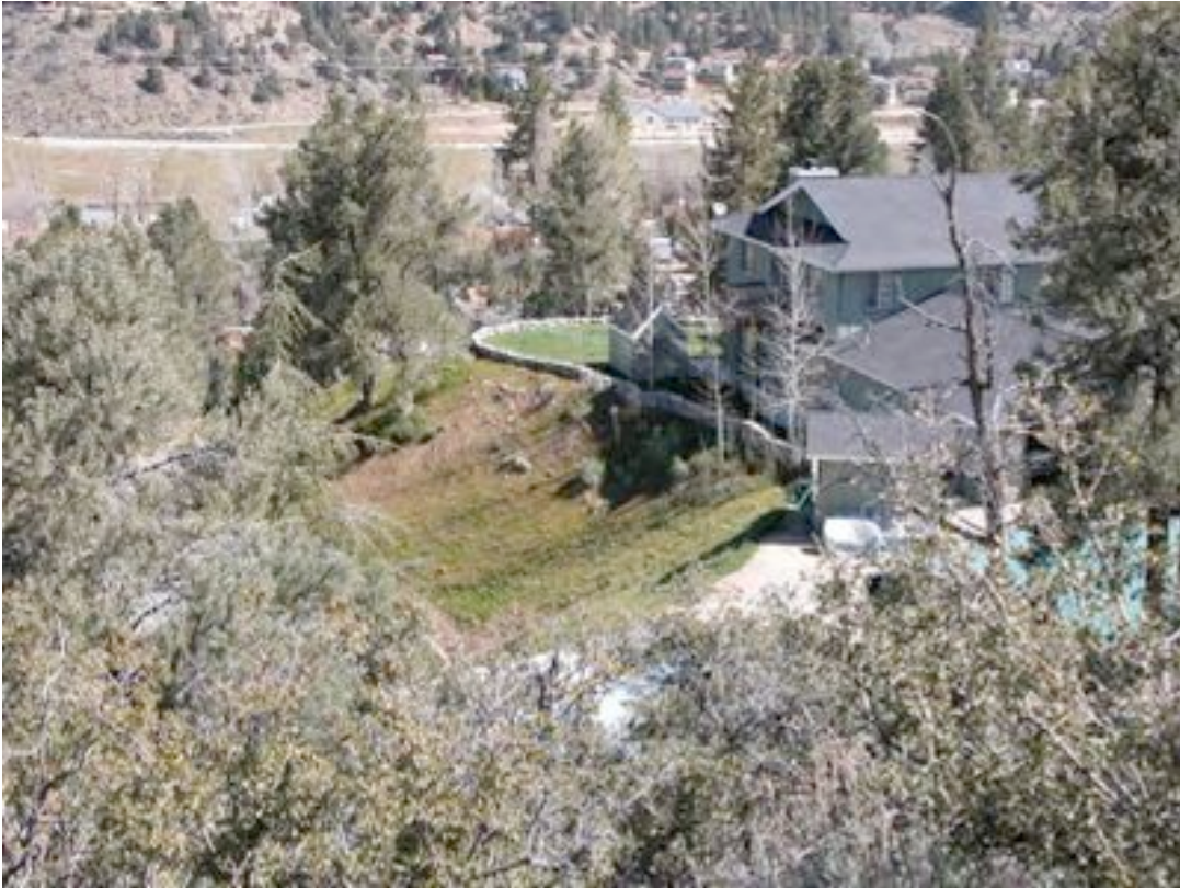
Figure 29: This home within the study area has provided defensible space by reducing the fuel load and irrigating the soil below the structure.
