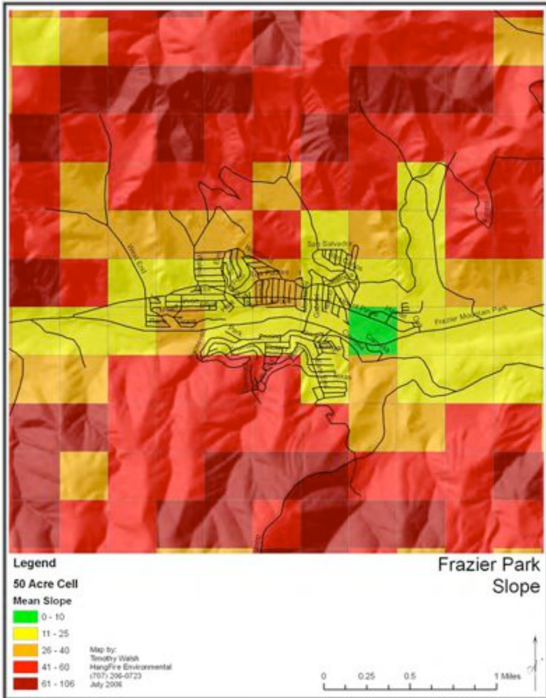
Map 18: The mean percentage of slope for each 50-acre cell in Frazier Park area.
