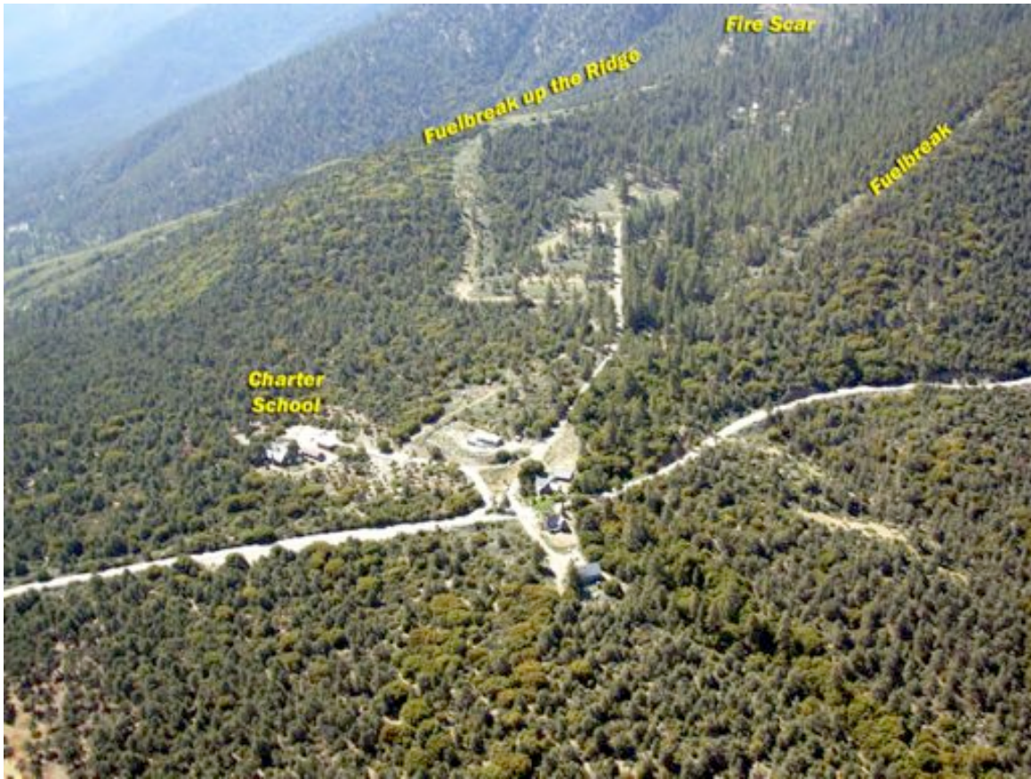
Figure 52: This image shows many different fuel modification strategies. In the center of the photo, the thinning around the Charter School can be seen. In the center of the photo, a fuelbreak runs up a ridge and ties into an old fire scar. Lastly, there is a fuelbreak in the upper right of the photo that continues upslope and stops. This fuelbreak should continue across USFS land and tie into a proposed fuelbreak in Block B of the Pine Mt. Club Project discussed earlier in this plan.
