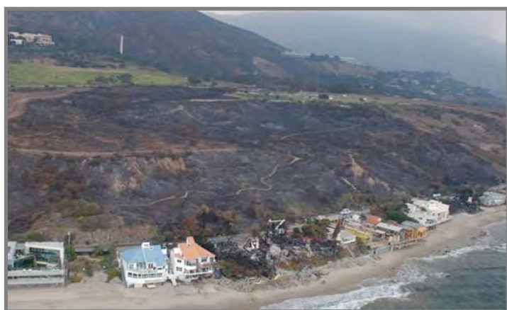
The Malibu Bluffs fire is an example of house-to-house combustion. Note there is still green vegetation surrounding the burnt houses. Source: Los Angeles Times
