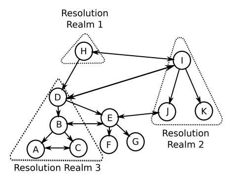
FIGURE 5.1. A Compass resolution overlay. CDAs with a double-arrowed link between them form a peer-to-peer relationship, but otherwise a customer-provider relationship. It has three content resolution realms, with each realm storing the resolution information for the entire content-ID space, while four CDAs are not part of any realm.
