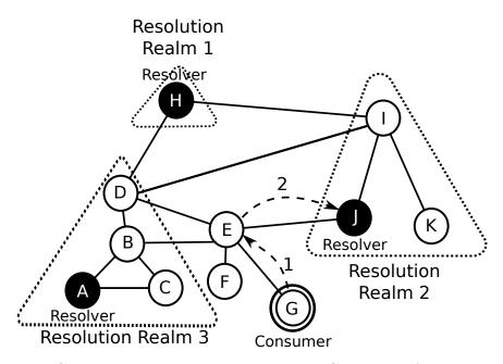
FIGURE 5.4. Content-ID resolution operation in Compass. A resolution request originates from CDA G and is forwarded via CDA E toward CDA J, which is the closest resolver to the consumer.
