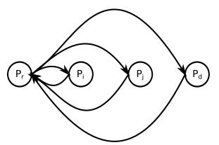
FIGURE 2.1. Iterative Routing Process in DHTs.
