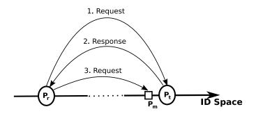
FIGURE 3.1. Message exchanges for adding a monitor and capturing destination traffic
