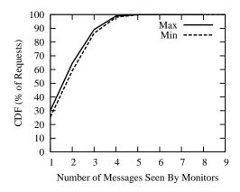
FIGURE 3.3. Routing Overhead in Kad
