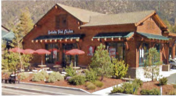
This fast-food restaurant has a gabled roof. The L-shaped footprint and the intersecting roofs of the two wings result in gable ends on multiple sides, which contribute to a varied roof line. The awnings attached to the building facades further break up the building scale and create visual interest.
