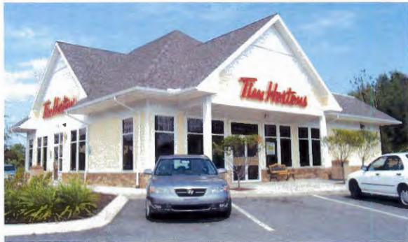
This small-footprint fast-food restaurant has a hipped roof. The roof line is broken up by gable ends that emphasize the building entries.
