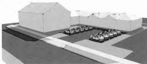
While off-street parking is typically preferred behind the building, this sketch illustrates how parking in the front may be permitted as long as at least 50 percent of the building's frontage complies with the maximum front setback.
