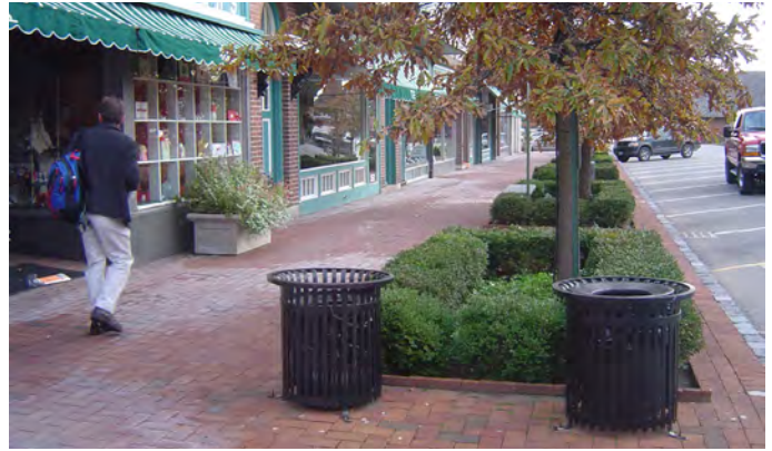
These trash containers have been placed in a furnishing zone outside the main pedestrian walking zone.
