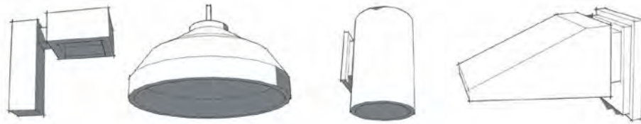
Figure 12.65.240-B: Examples of Shielded Light Fixtures
