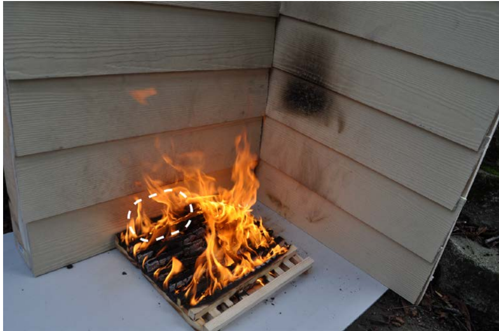
Figure 10 Class "A" Brand Burning
