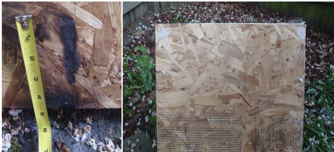
Figure 11 Control wall Sheathing (left) and rainscreen sheathing (right)
