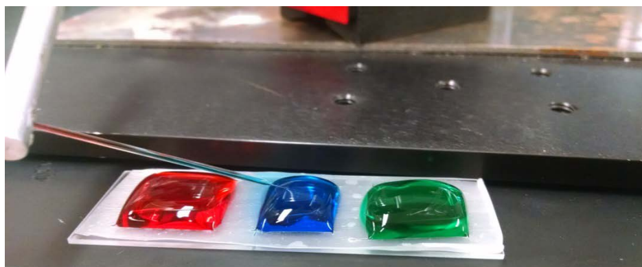
Figure 10: Three-Well Chamber for Filling Pipettes
