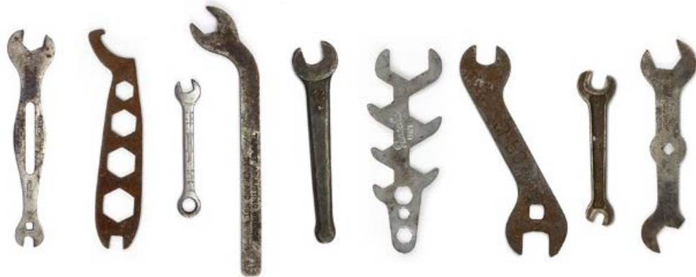
Figure 15. A sample of wrenches illustrating stylistic modes that vary from wrench to wrench (e.g., composing metal) and functional modes that are shared by all (e.g. hexagonal notch). Source:“Wrench.” The Typology . Diana Zlatonovski. 2010-2013. Web. 20 May 2015.
