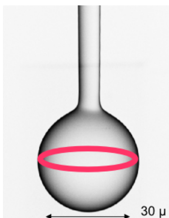
FIGURE 3.2. Image of a microsphere, with the path of the optical cavity drawn for clarity. Note the presence of the stem, which is how the sphere is held in place.
