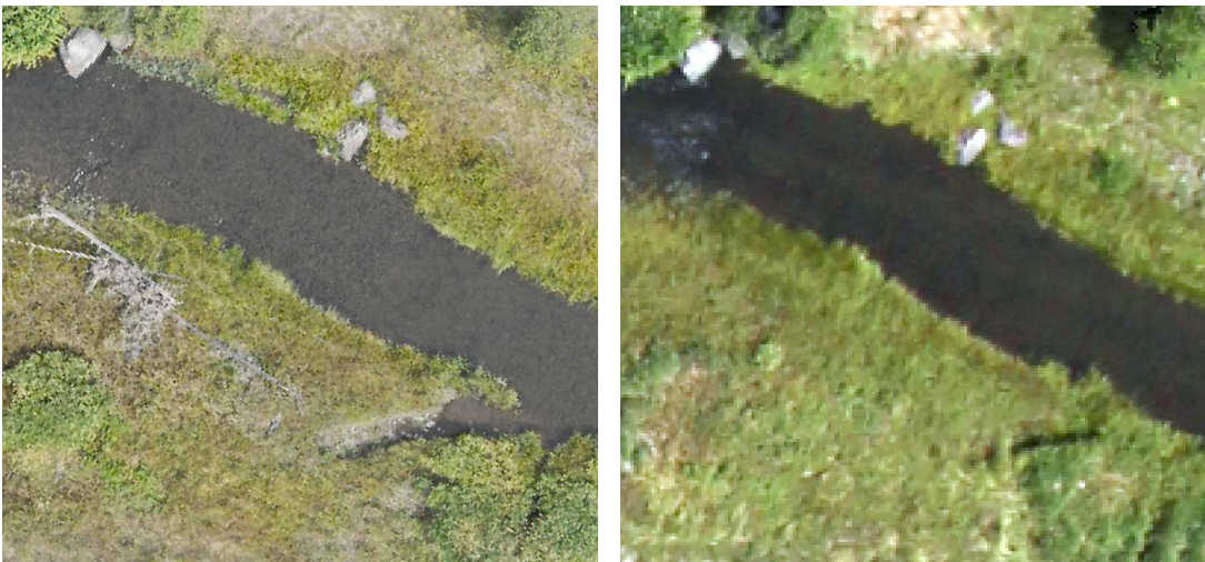
Aerial photos of VIBR log structure 10 . Photo from 2009 is on the left and 2013 is on the right. This log structure was completely washed away and the alcove has been filled.
