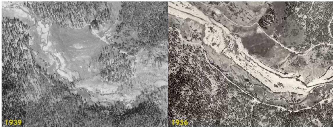
Figure 3: River channel pre and post dredge mining. In 1939 the channel meanders along the southern part of the floodplain. After dredge mining (1956) the channel is left abandoned and the channel runs straight alongside the tailing piles, which are the white areas. Source: Bureau of Reclamation 2008a.
