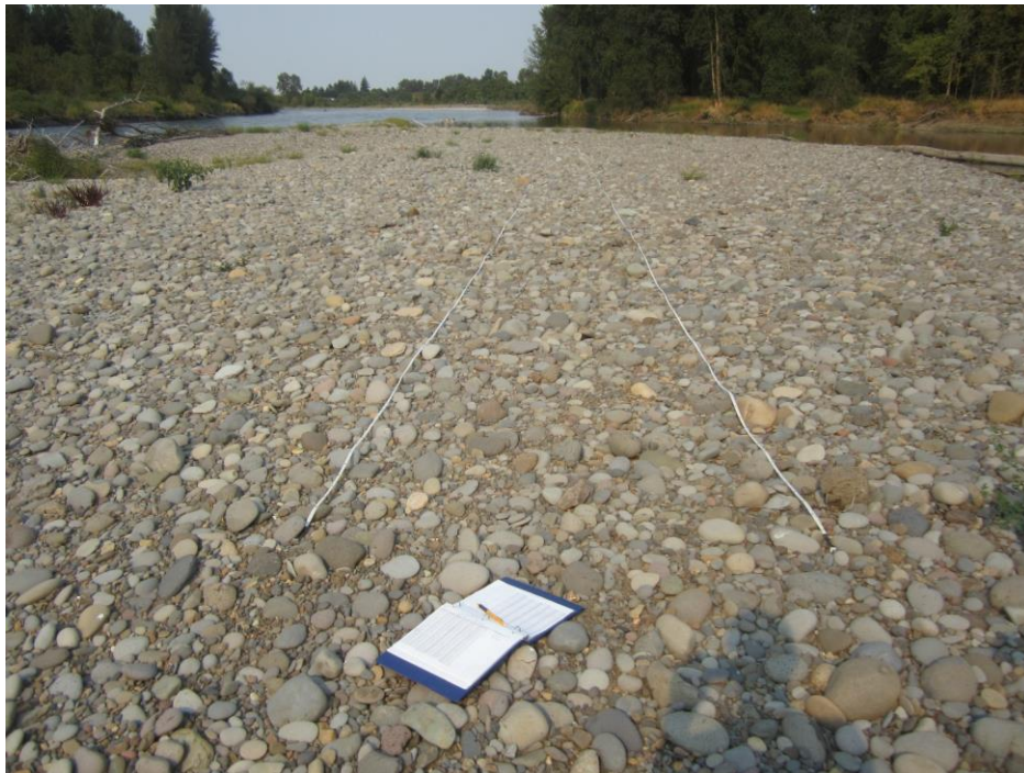
Figure 5. Sampling setup for grain size measurements. Photograph taken at Bar 4.
