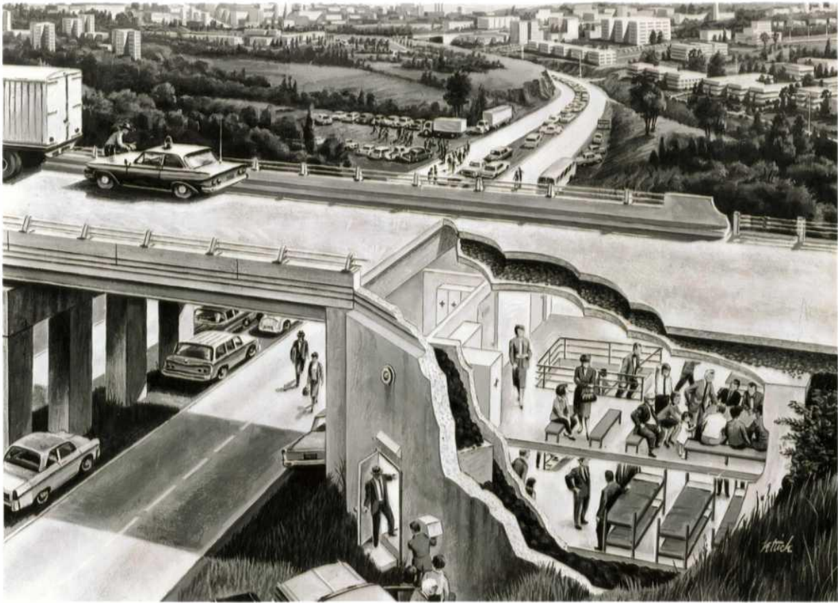
Fig. 1: A prototype highway shelter as envisioned by federal Civil Defense officials. Photo # 311-M-23-9, Record Group 311, Still Pictures Branch, National Archives, College Park, MD. Courtesy David Monteyne, University of Calgary.
