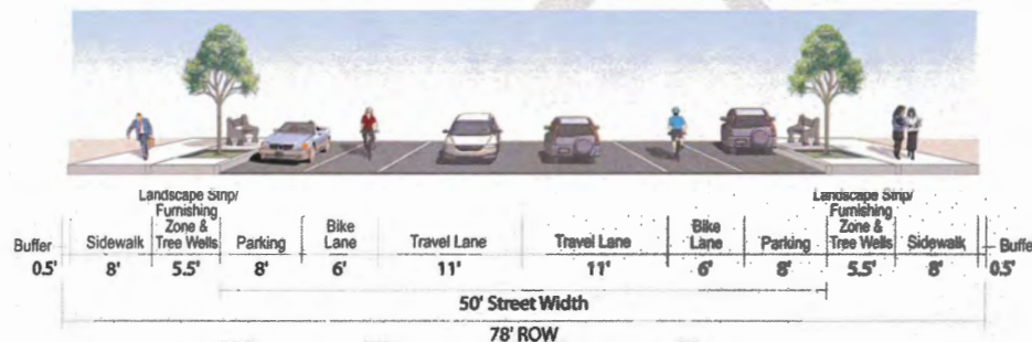
Figure 18.660.7 Cross-Section for Collector within Community Commercial Zone
