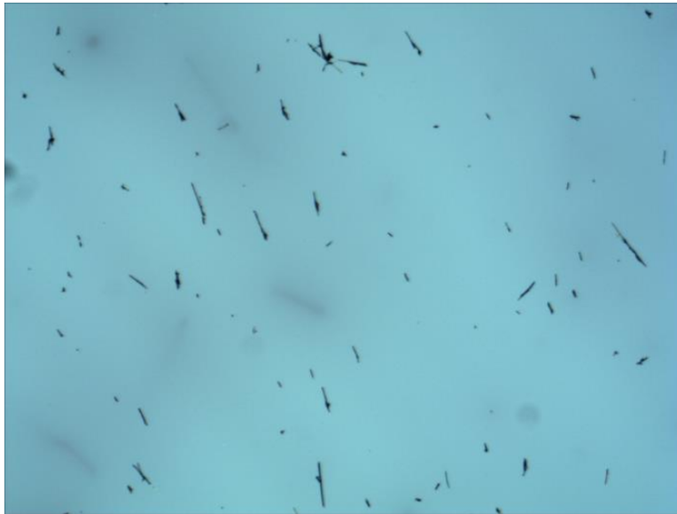
Figure 3.9. Optical image (100x magnification) of tungsten oxide nanowires deposited on SiO 2 substrate from EtOH suspension.
