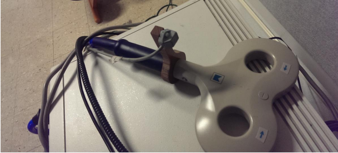
Figure 6.1. The sensor attached to the coil with a customized bracket.
