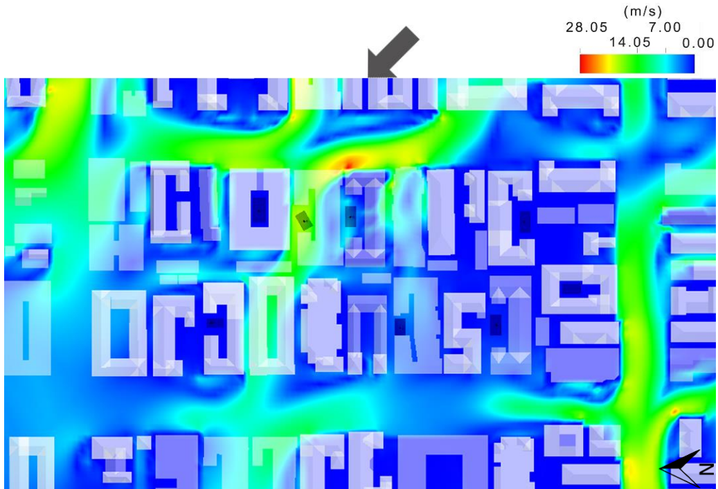
Fig. 49. Courtyard houses, simulation for oblique wind of 2.5 m/s. Autodesk screen shot reprinted courtesy of Autodesk, Inc.
