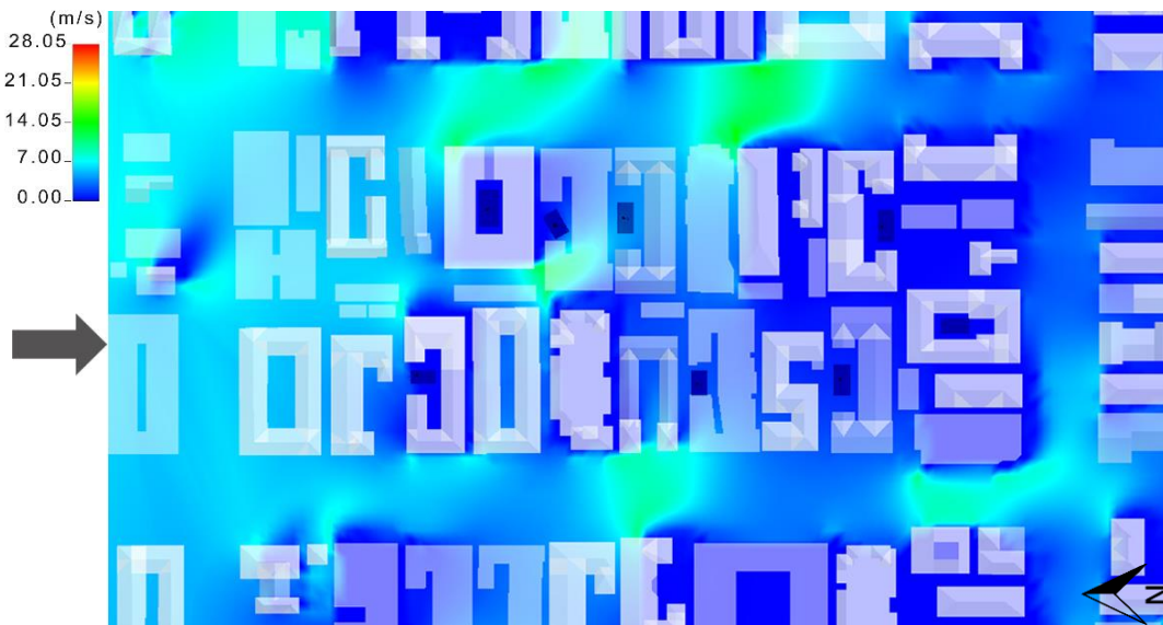
Fig. 46. Courtyard houses, simulation for parallel wind of 5.5 m/s. Autodesk screen shot reprinted courtesy of Autodesk, Inc.
