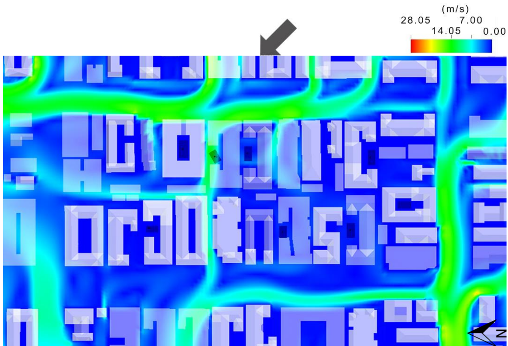
Fig. 50. Courtyard houses, simulation for oblique wind of 5.5 m/s. Autodesk screen shot reprinted courtesy of Autodesk, Inc.
