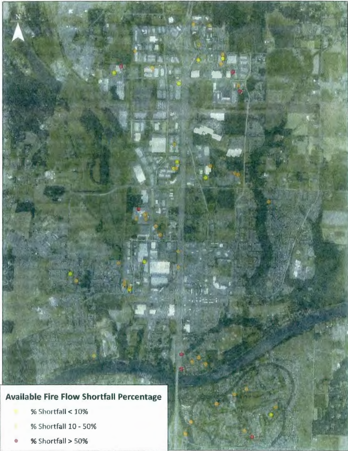
CHART 3.1 - Wilsonville Localized Fire Flow Deficiencies
