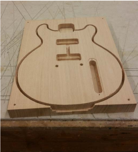
Guitar blank after the CNC cut.
