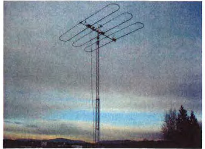
Directional beam antenna
