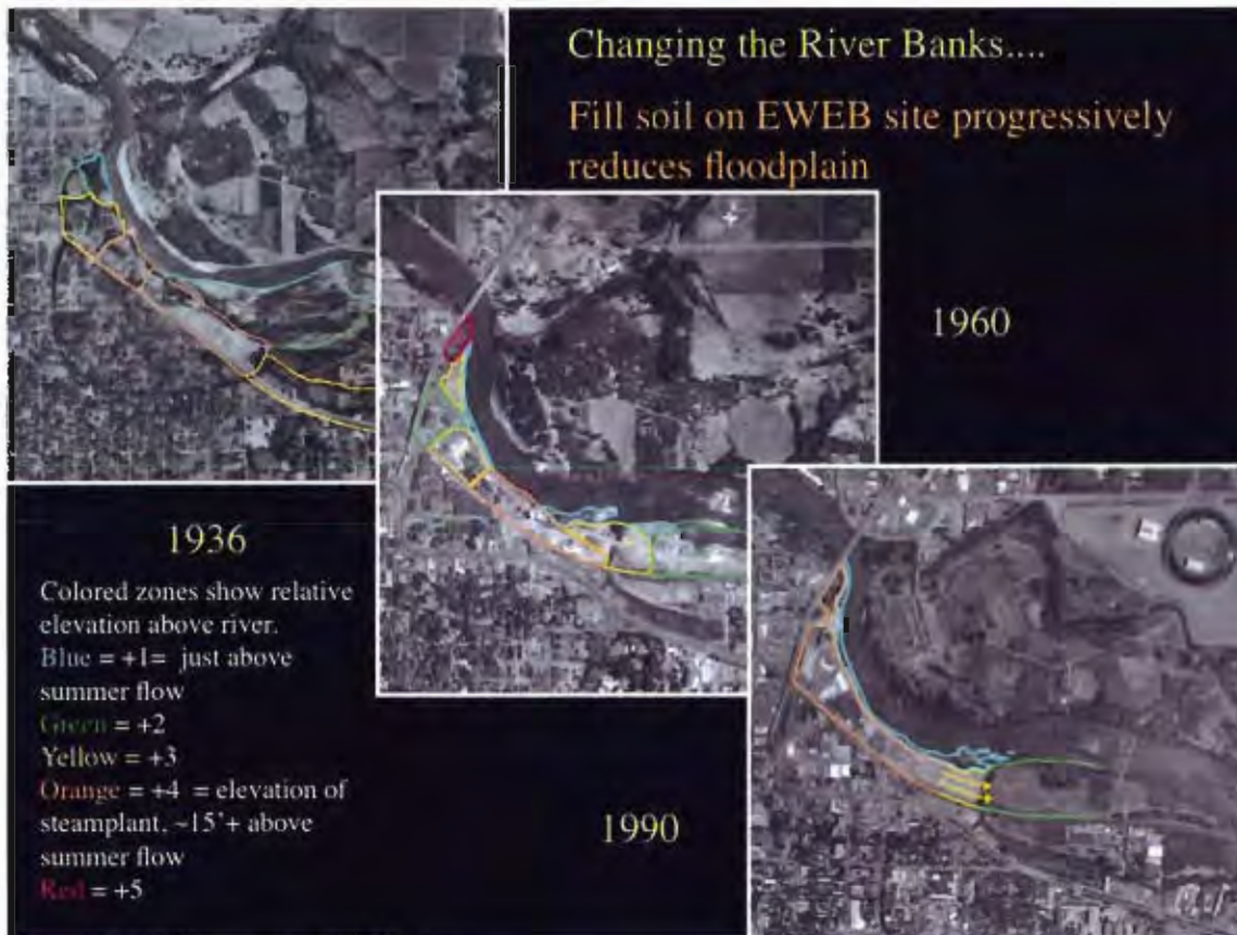
Figure 13. Fill Placement on EWEB site.
