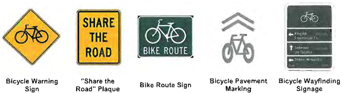
Figure 6-45 Bicycle Signs and Markings
