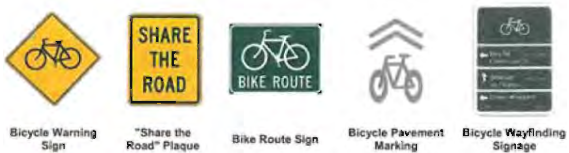
Figure 6-5 Bicycle Signs and Markings
