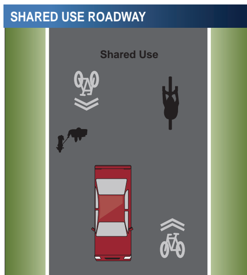
Note: Functional for low speed, low vehicle traffic roadways.
