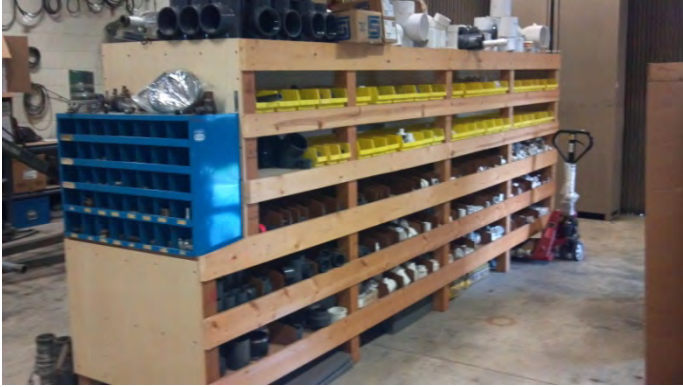
Figure 7 .Storage Rack Requires Bracing
