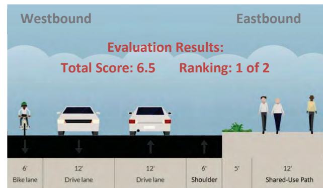
Option 2: Widen roadway to provide bike lanes and a shared-use path
