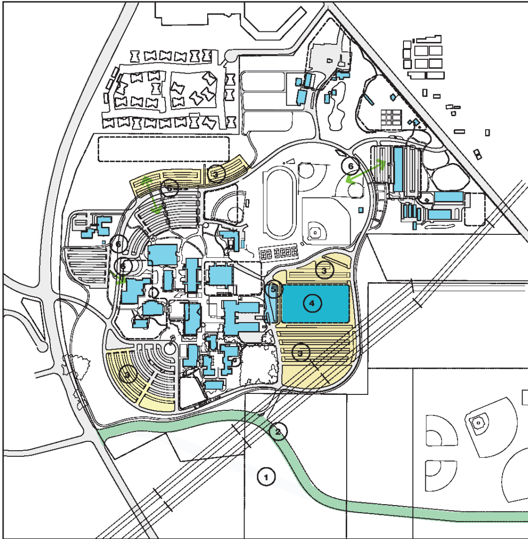
Figure 7. Potential Future Access and Parking Improvements
