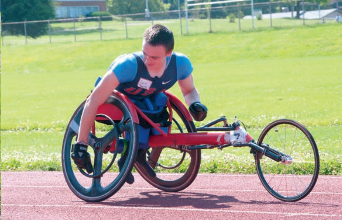
Abbott demonstrates a proper stroke from his glove to the pushrim of his racing chair. Wheelchair athletes wear gloves with fold-over grip pads to protect their hands while powering their three-wheeled racers.
