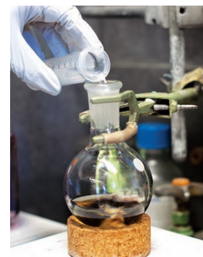
A reduction of gold salts changes the color of the solution to deep purple as the size and properties of the nanoparticles change.
